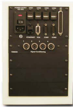
Typical EPIC-CAG side panel with 4-channel signal conditional cards.
