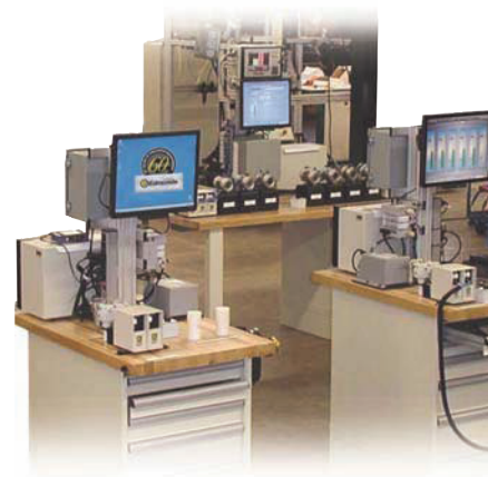
EPIC-CAG configured as an inspection station.
